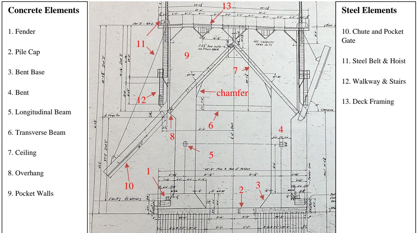
Figure 1: Section View of Bent.
