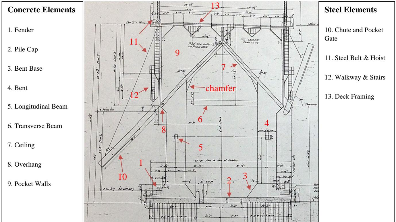
Figure 1: Section View of Bent.
