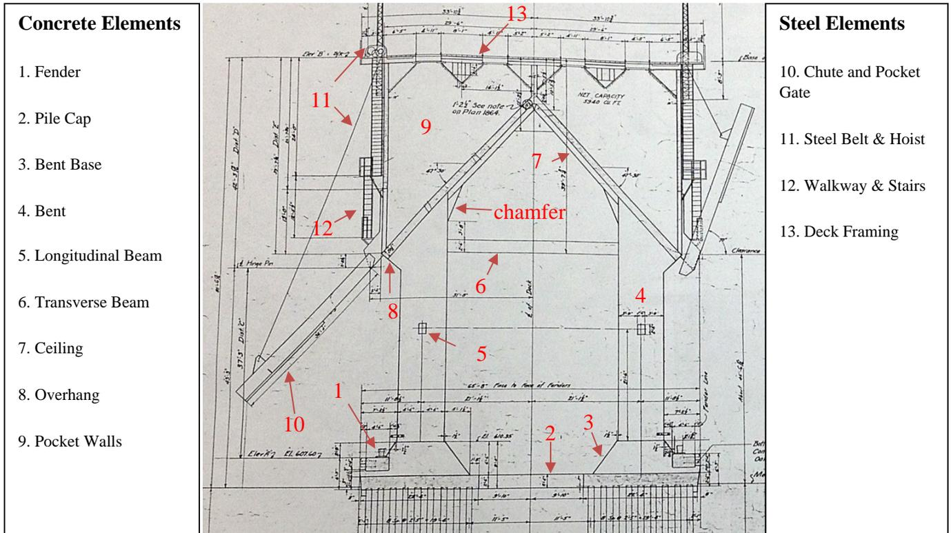
Figure 1: Section View of Bent.
