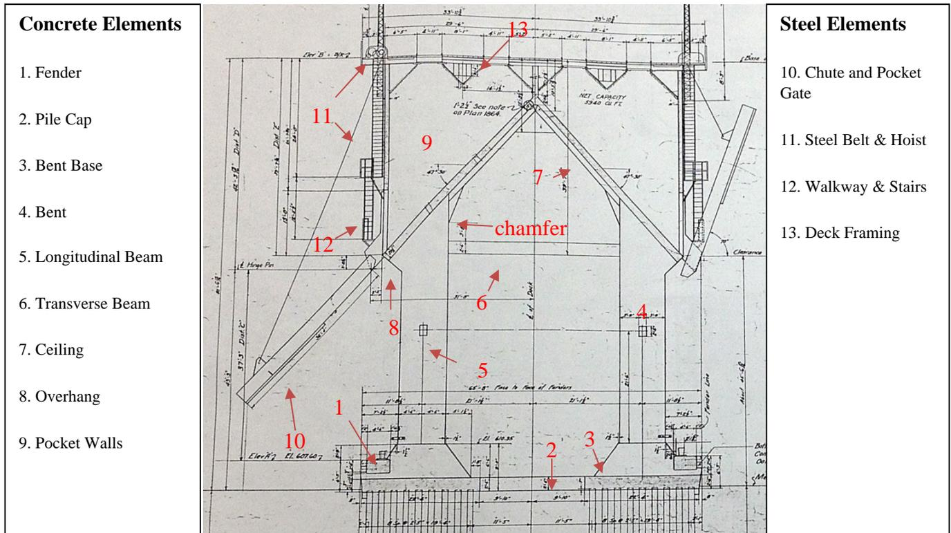
Figure 2: Section View of Bent.
