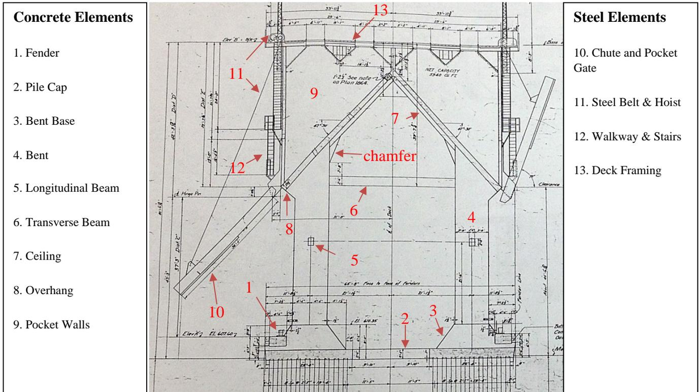
Figure 1: Section View of Bent.
