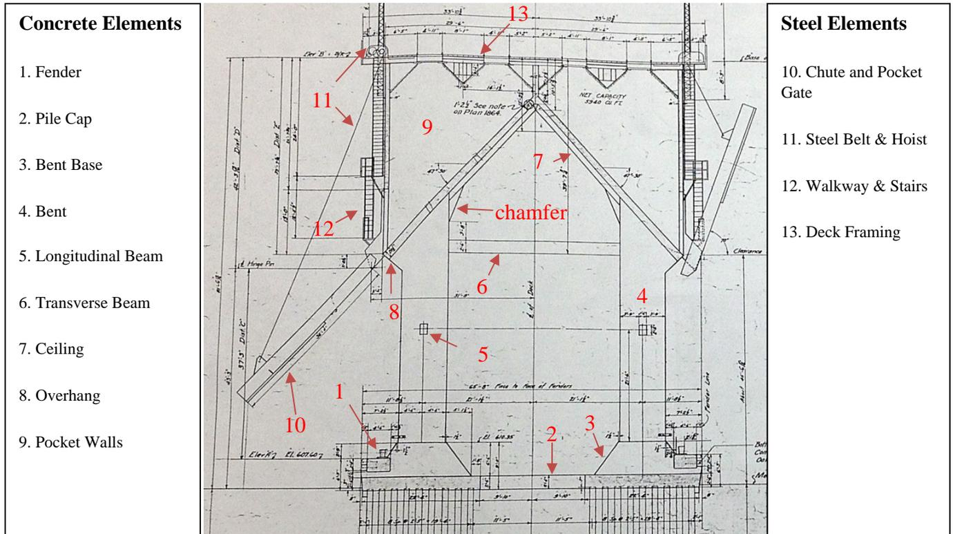
Figure 1: Section View of Bent.
