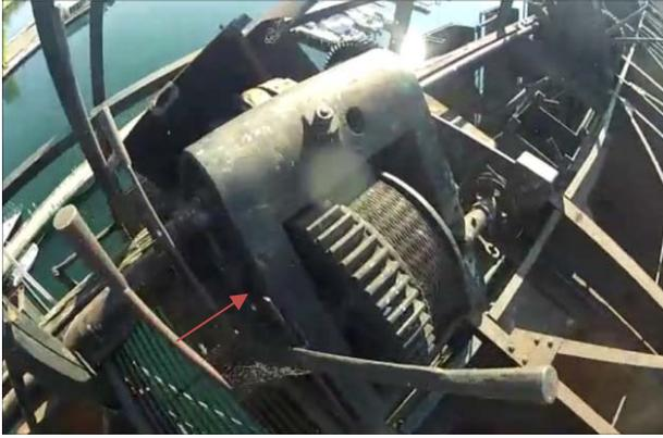
*Photo 3-19: View of typical hoist showing various levers used to operate the chutes and pocket gates. Note lever used to lock chute belt real into place.*
