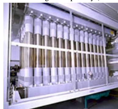
Continuous Microfiltration Units
