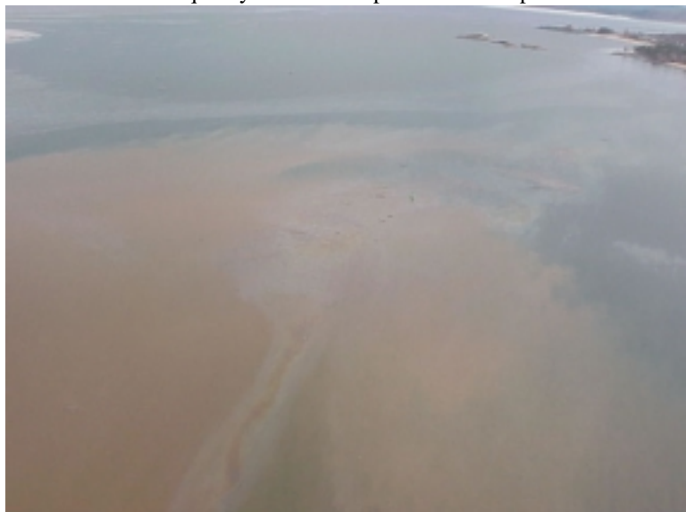
Sediment and Oil Plume in Marquette WTP Source Water Area Resulting from Dead River Dam Failures (May 15, 2003 Photo from city of Marquette Website)
