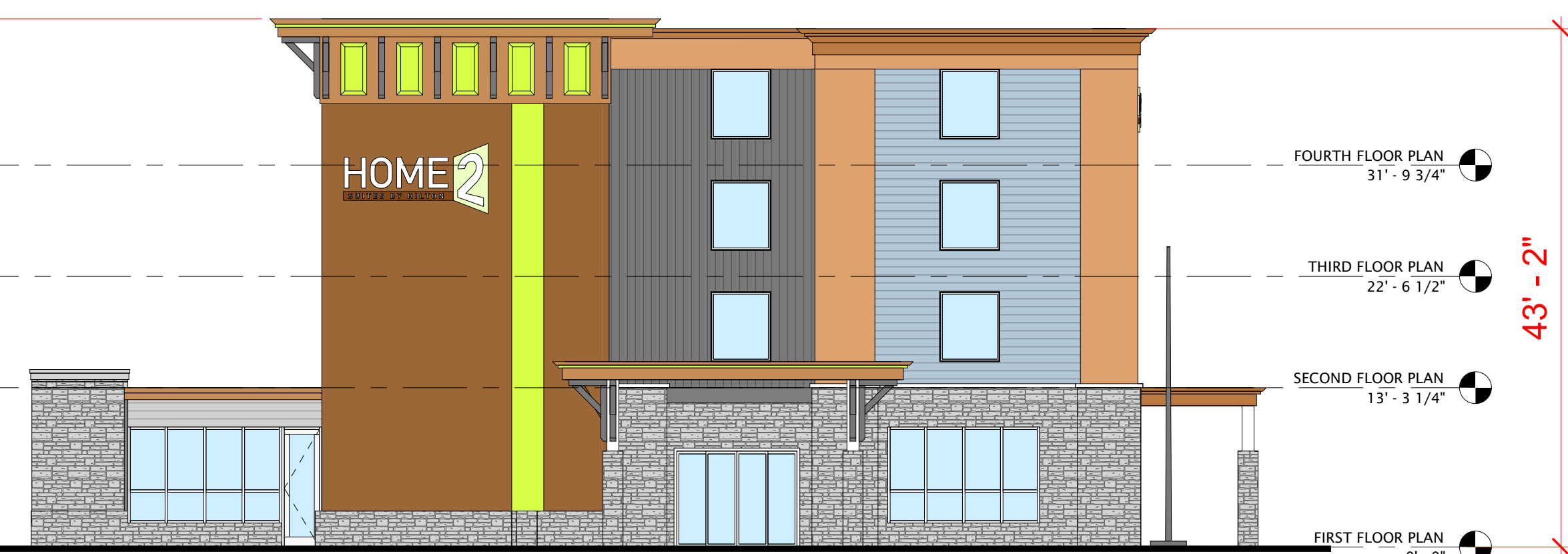
SOUTH EXTERIOR ELEVATION 3/32" = 1'-0"
