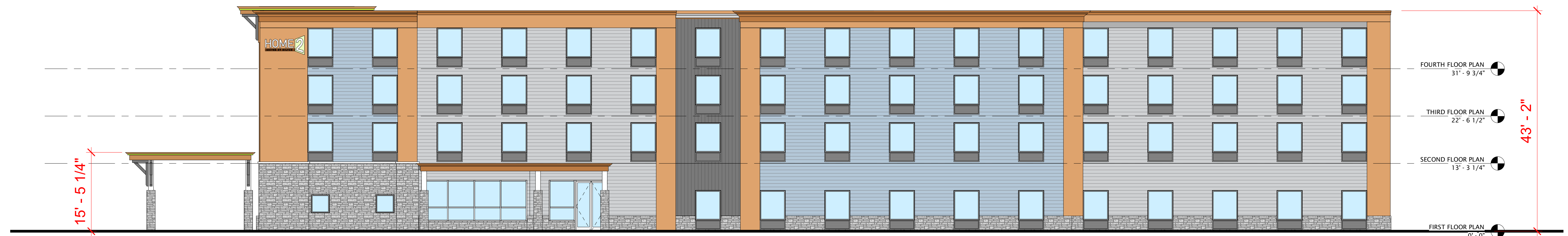
EAST EXTERIOR ELEVATION 3/32" = 1'-0"
