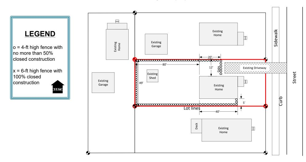
The drawing must indicate the location of the proposed fence in relation to all **property lines**, **adjacent structures**, **zoning districts**, **and street corners**. **The dimension of the fence lengths will need to be also shown**. (An air photo may be obtained for a fee from the Community Development Department for this purpose)
