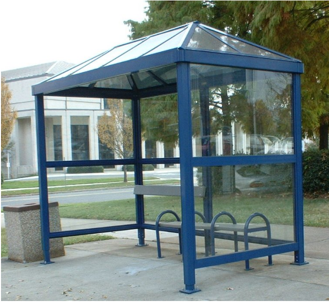
Figure 20: Brasco 5' x 10' shelter with tinted acrylic hip roof, powder coated blue. Charlotte NC. Cost: about $5,000, not including installation, concrete pad, power, bike rack (not shown) trash receptacle
